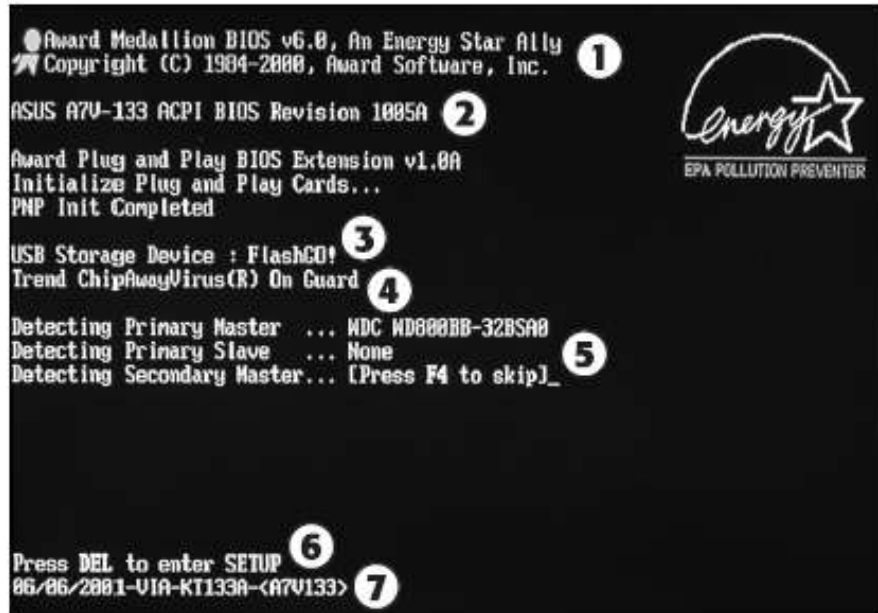
FIGURE 2.24 A typical startup screen displaying detected drives, chipset, and BIOS information.
